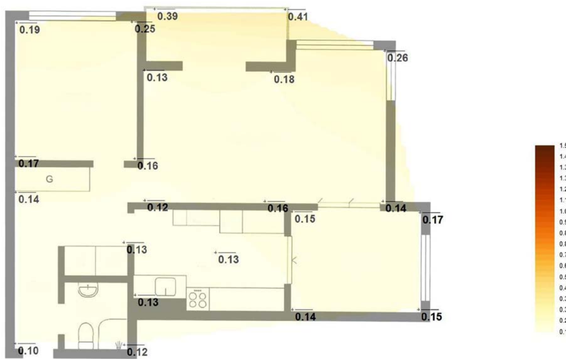
Figure 7. Spatial field distribution map of the low exposure apartment; time-averaged RF electric field ( \text{V m}^{-1} ). RF, radiofrequency.
