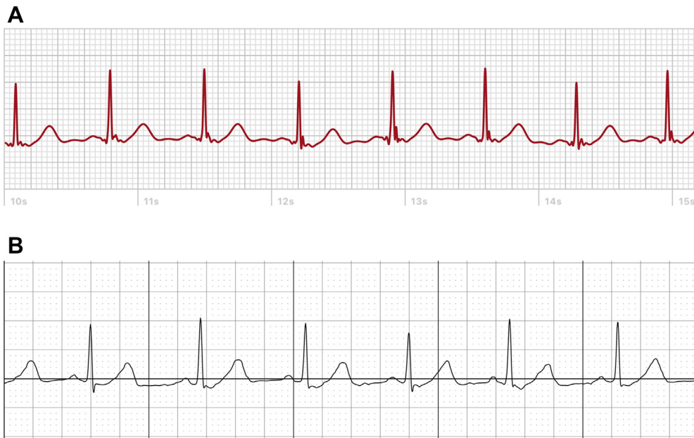
Figure 3 A: Apple Watch (Apple, Cupertino, CA) tracing performed with deep brain stimulator on reveals no identifiable electrogram artifact. B: KardiaMobile 6L (AliveCor, Mountain View, CA) tracing obtained in single-lead mode also reveals no evidence of identifiable electrogram artifact. This holds true for 6-lead mode as well.
