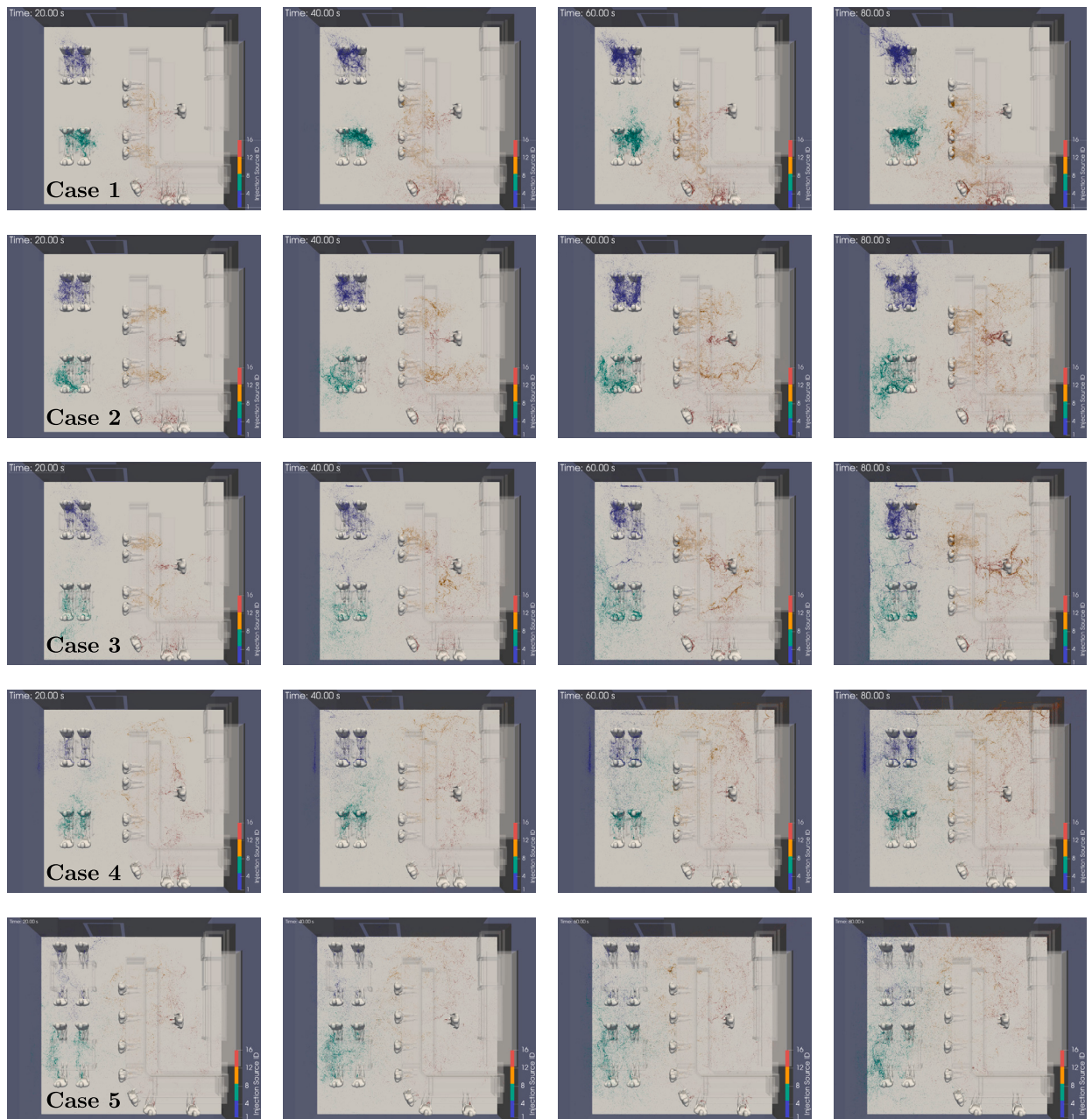
Fig. 6. Snapshot of droplet dispersion at time instants 20 s, 40 s, 60 s and 80 s of Cases 1 to 5. The top row of images correspond to Case 1, the next row to Case 2, on and the bottom row to Case 5.
