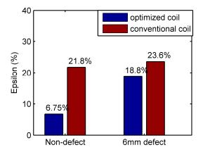
**Figure 15.** Experimental Results—Comparison of reduction in *c* of the conventional coil and optimized coil for centered and off-center rivets.
