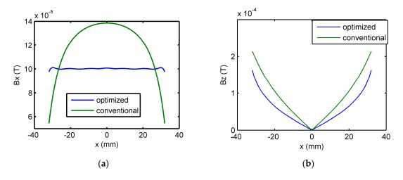
**Figure 7.** Numerical simulation results of (**a**)  $B_x$  at the observation points and (**b**)  $B_z$  at the sensor array for the cases of optimized coil and uniform coil.
