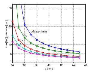
**Figure 5.** Calculation results:  $\eta$  vs. parameter "*a*" for different air gap width w<sub>air</sub>.
