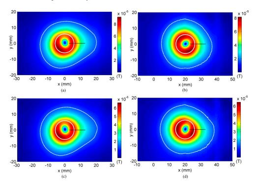
**Figure 10.** Simulation results for cases: (a) conventional coil, rivet center located at x = 0 mm; (b) conventional coil, rivet center located at x = 20 mm; (c) optimized coil, rivet center located at x = 0 mm; (d) optimized coil, rivet center located at x = 20 mm.
