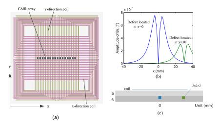
**Figure 1.** (a) Top view of orthogonal coils and linear array sensors; (b) Simulation result of response signals due to defect located at x = 0 mm and x = 30 mm; (c) Lateral view of the model.
