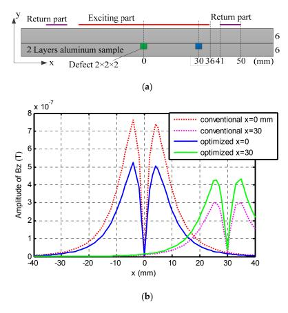
**Figure 8.** (a) Lateral view of tested sample and excitation coil; (b) Simulation results of the optimized coil and uniform distribution coil for a defect located at x = 0 mm and x = 30 mm after background subtraction.
