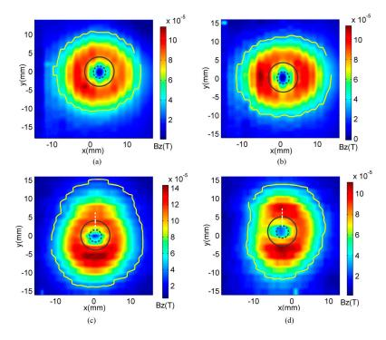
**Figure 14.** Experiment results of (**a**) defect free rivet generated using optimized coil; (**b**) defect free rivet generated using conventional coil; (**c**) rivet with a 6 mm length 2nd layer defect generated using optimized coil; (**d**) rivet with a 6 mm length defect generated using conventional coil.
