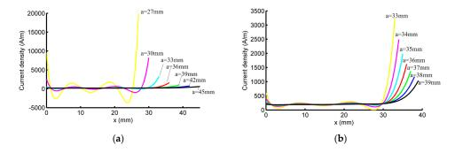
**Figure 3.** Optimization result: current density distribution vs. *x* for different values of parameter "*a*". (a)  $27 \le a \le 45$ ; (b)  $33 \le a \le 39$ , which is the possible range of "*a*" for optimized probe.
