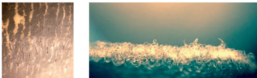
Figure 5. Results from composite-to-sheath bonding evaluations. Left: Nylon sample showing delamination. Right: Edge of cotton sheath showing composite sitting on top of the cotton rather than encapsulating the cotton fibers.
