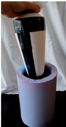
Figure 6. Magnetic composite sheath formation. A coated sheath on a foam positive about to be inserted into the negative mold.
