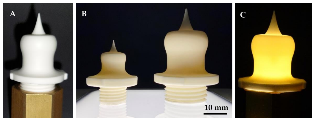
Figure 15. A 10 N nozzle within a metallic counter thread (A); visualization of the size difference (B); transillumination by lamp for (large) defects (C).
