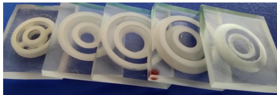
Figure 13. Test specimen embedded in epoxy resin and cut into segments.
