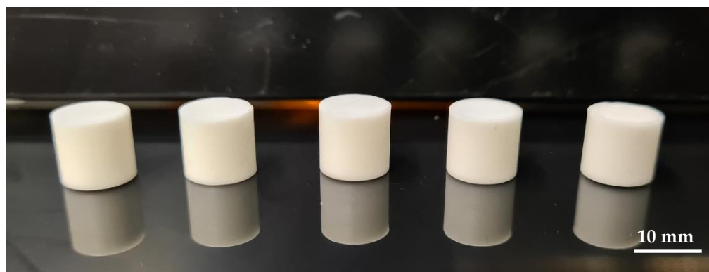
Figure 7. Sintered alumina cylinders ( d = 12 mm) based on suspension rc3.
