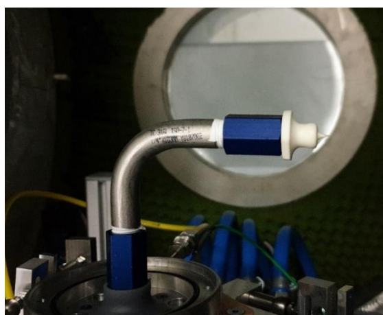
Figure 17. Vacuum test bench for characterization of nozzle flow characteristics; equipped with 2.5 N nozzle.
