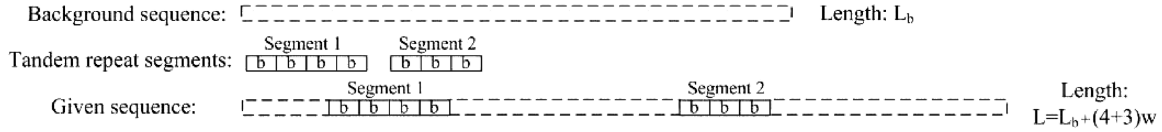
Figure 1. A schematic view of a sequence with DSATR. A background sequence and multiple repeat segments are generated independently. All repeat units in these repeat segments are random instances of a common motif ‘b’ of width w . The input sequence is generated by randomly inserting the repeat segments into separated locations in the background sequence.
