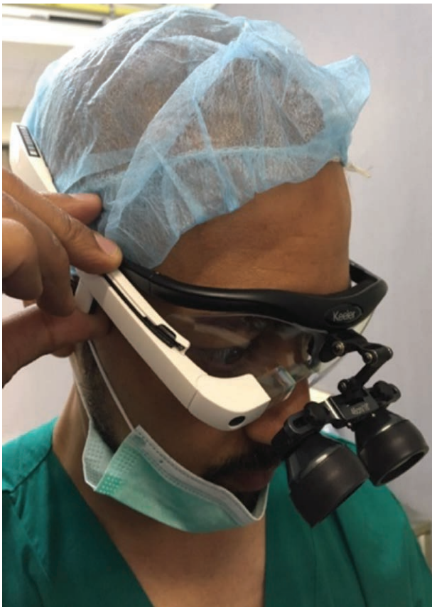
Fig. 5. Fitting the Google Glass headset over surgical loupes.
