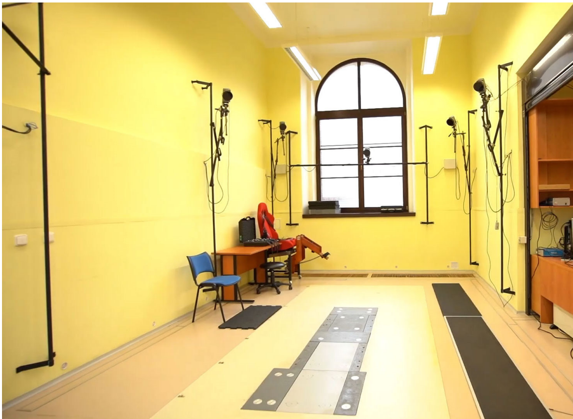
Figure 1. The specialized laboratory with 5 of the 11 infrared cameras Oqus 300 and 300+ visible, placed along the laboratory walls and 2 force platforms (light grey rectangles) placed on the laboratory floor.
