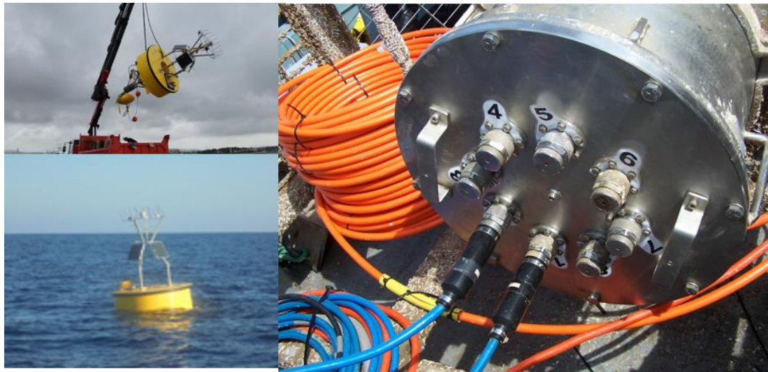
Figure 3. The used moored surface buoy (on the left) and depth-rated SP junction box (on the right) for motherboard processing and sensors connections.
