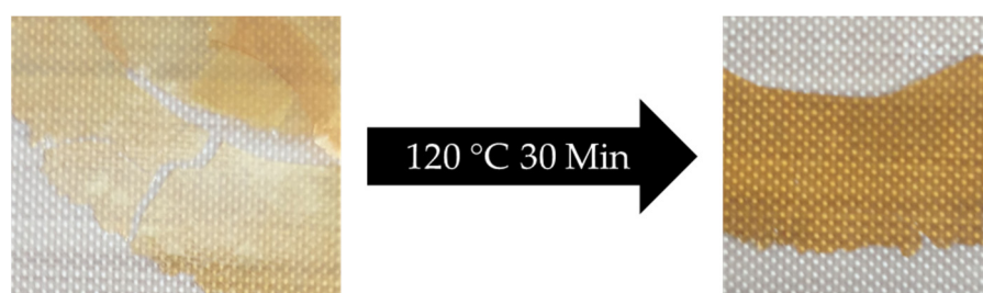
Figure 13. Reshaping of cracked P(BA 60-co -FMA 40 ) 10 crosslinked with BMI with a motif ratio of 1:1 at room temperature. Broken polymeric film on the left side and cured polymeric film on the right side .
