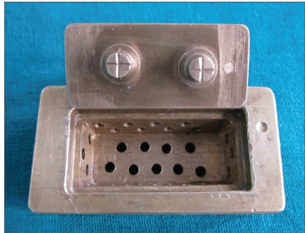
Figure 2: Brass master die and perforated stock tray
