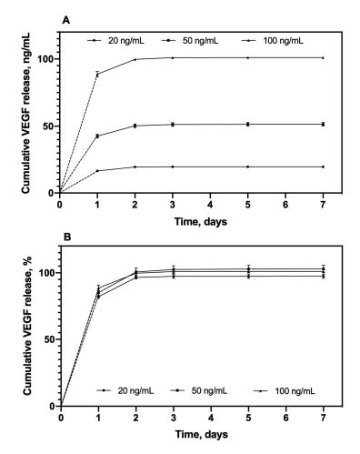
**Figure 7.** In vitro cumulative release profiles expressed (**A**) in ng/mL and (**B**) as percentage of CHT/PCD sponges loaded with 20, 50, and 100 ng VEGF in ECM culture medium supplemented with 0.5% FCS at 37 °C under static conditions. The test was repeated twice and each in triplicate (n = 6).
