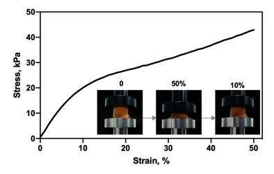
**Figure 5.** Compressive stress–strain curve of CHT/PCD sponge after immersion in PBS for 2 h, tested at room temperature. Representative images of sponge during the compression test. On the left, the scaffold at the beginning of the test; in the middle, scaffold compressed at 50% strain; on the right, scaffold recovered their shape at the end of the test (10% strain). The curve corresponds to the average values of three repetitions (n = 3).
