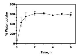
**Figure 3.** Water uptake profile of CHT/PCD sponge in PBS (pH 7.4) at 37 °C and 80 rpm. The test was carried out at least twice and each in triplicate (n = 6).
