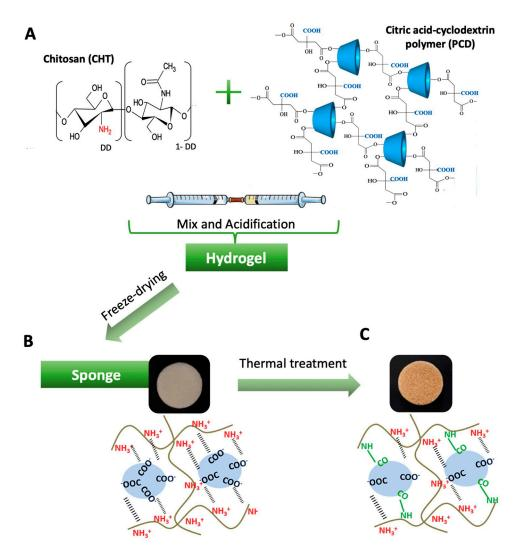
**Figure 1.** Schematic representation of the formation of chitosan/*anionic* cyclodextrin polymer (CHT/PCD) 3:3 sponge. (A) Chemical structure of CHT and PCD and the double-syringe system used for the obtaining of hydrogel. Macroscopic observation of sponge and the molecular interactions between CHT and PCD (B) after freeze-drying and (C) after thermal treatment.
