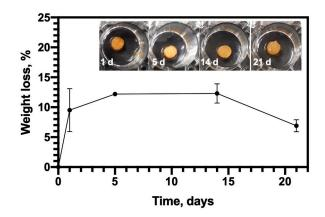
**Figure 4.** Biodegradation of CHT/PCD sponge (expressed in percentage of weight loss) in PBS (pH 7.4) supplemented with 0.5 mg/mL lysozyme at 37 °C and 80 rpm and representative images of scaffolds removed after each time point up to 21 days. The test was carried out at least twice and each in triplicate (n = 6).
