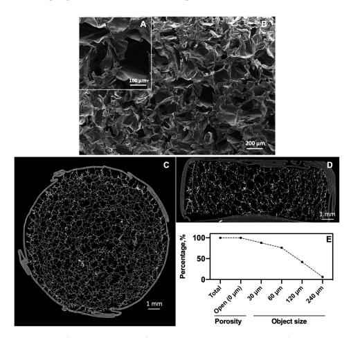
**Figure 2.** Analysis of the microstructure of the CHT/PCD sponge. SEM images of the cross-section of the scaffold: (**A**) At  $\times$ 50 and (**B**) at  $\times$ 100 magnification.  $\mu$ CT cross-section images: (**C**) Horizontal view, (**D**) vertical view (both images show the parafilm layer used around the samples), and (**E**) percentage of available interconnected porosity to allow passage of an object of defined size into the scaffold.
