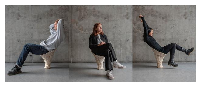
**Figure 15.** Seating tests (44 to 90 kilos).
