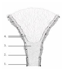
**Figure 10.** Section: 1. Rattan Ø 2 mm, 2. Rattan Ø 5 mm, 3. Mycelium substrate, 4. Hemp fibers.
