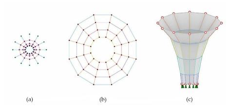
Figure 8. (a,b) Form and Force Diagram, (c) Thrust Diagram.
