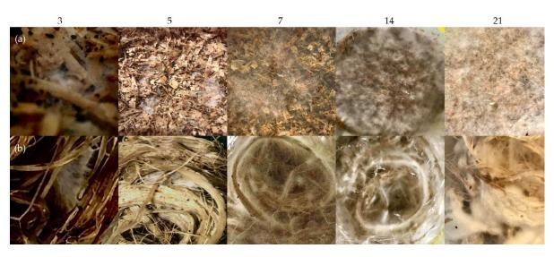
Figure 4. Growth process in days: (a) wood chips, (b) hemp fibers.
