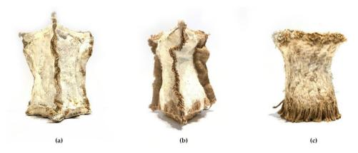
**Figure 6.** Results of grown on different skin materials: (a) hemp sheets, (b) jute sheets, (c) knitted hemp rope.
