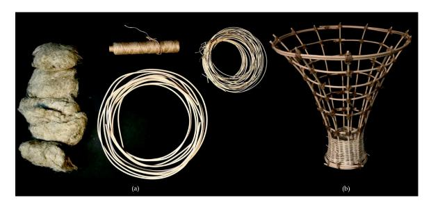
Figure 11. Material overview: (a) hemp fibers, rattan rods, jute fabric, (b) assembled rattan frame.
