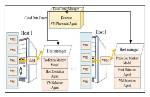
Fig. 5 Working section of VM (Manasrah et al. 2017)
