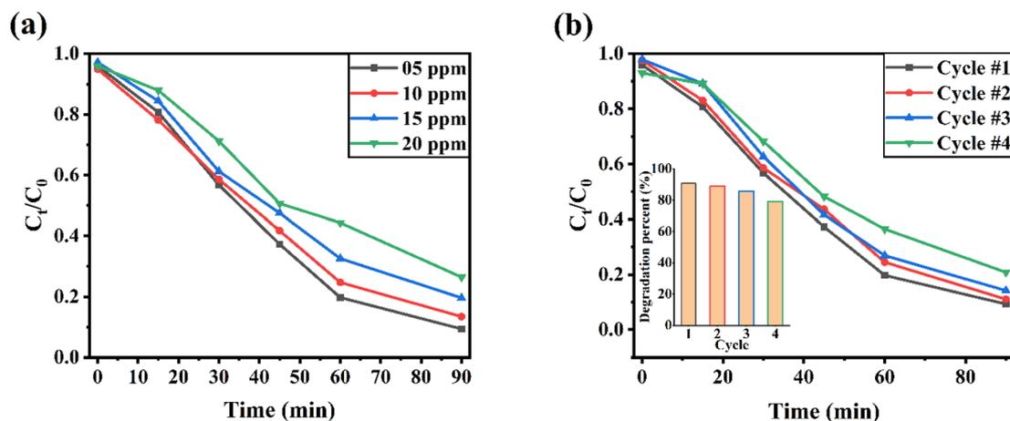
Fig. 9 (a) MB dye photodegradation efficiency with various concentrations in the presence of  $50 \text{ mg L}^{-1}$  of rGO/NiO<sub>x</sub>/Ag ternary composites. (b) The reusability MB degradation performance of rGO/NiO<sub>x</sub>/Ag system.
