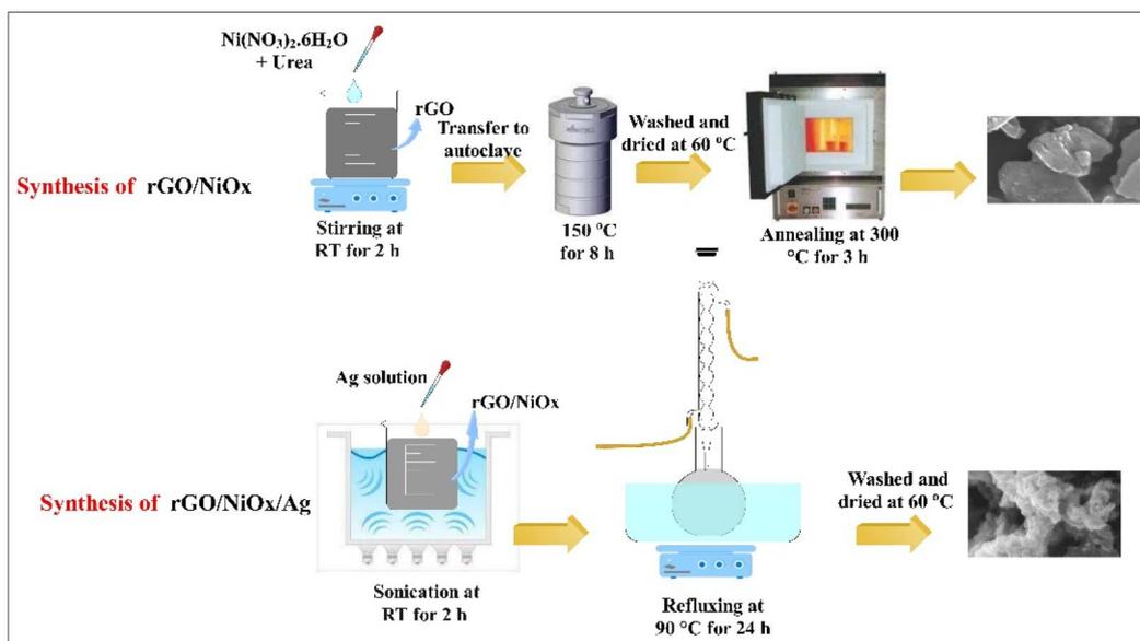
Fig. 1 Schematic diagram for synthesis of rGO/NiO<sub>x</sub> and rGO/NiO<sub>x</sub>/Ag materials.
