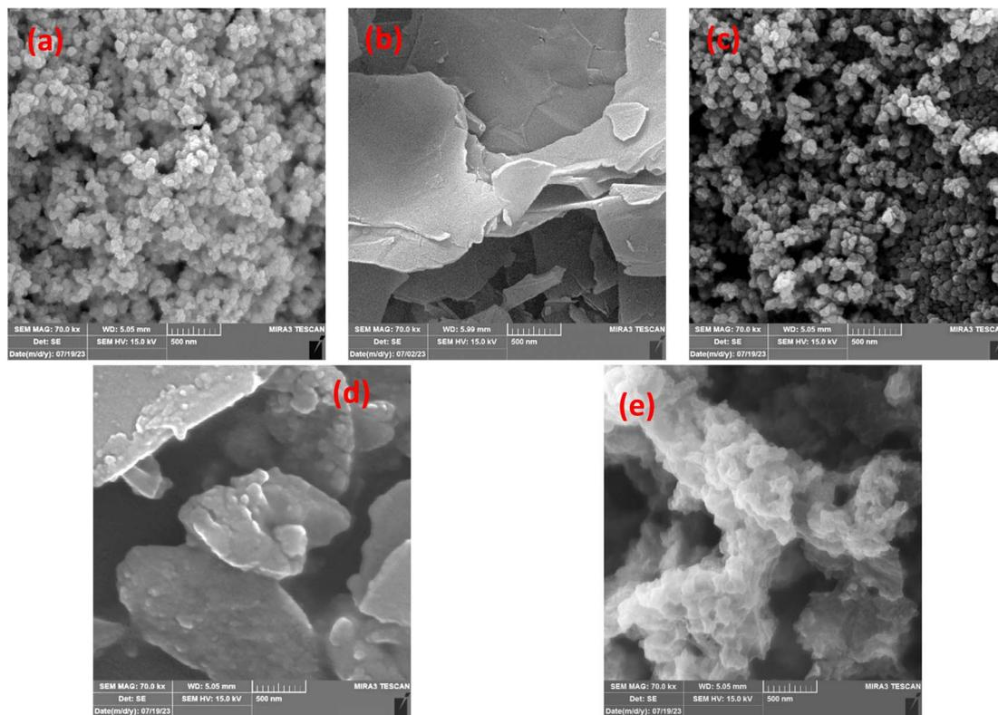
Fig. 4 FE-SEM image of (a) Ag nanoparticles, (b) rGO sheets, (c) NiO<sub>x</sub> nanoparticles, (d) rGO/NiO<sub>x</sub> composites, and (e) rGO/NiO<sub>x</sub>/Ag ternary composites.
