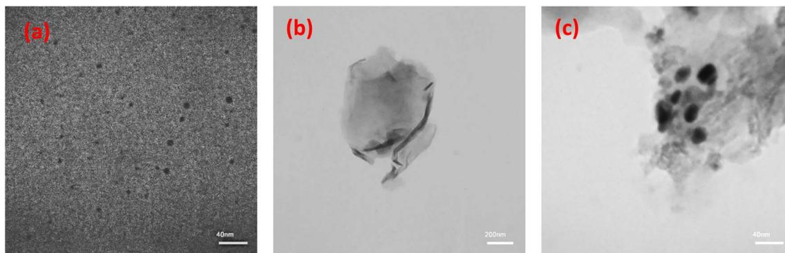
Fig. 6 TEM images of (a) Ag nanoparticles, (b) rGO sheets and (c) rGO/NiO<sub>x</sub>/Ag ternary composites.
