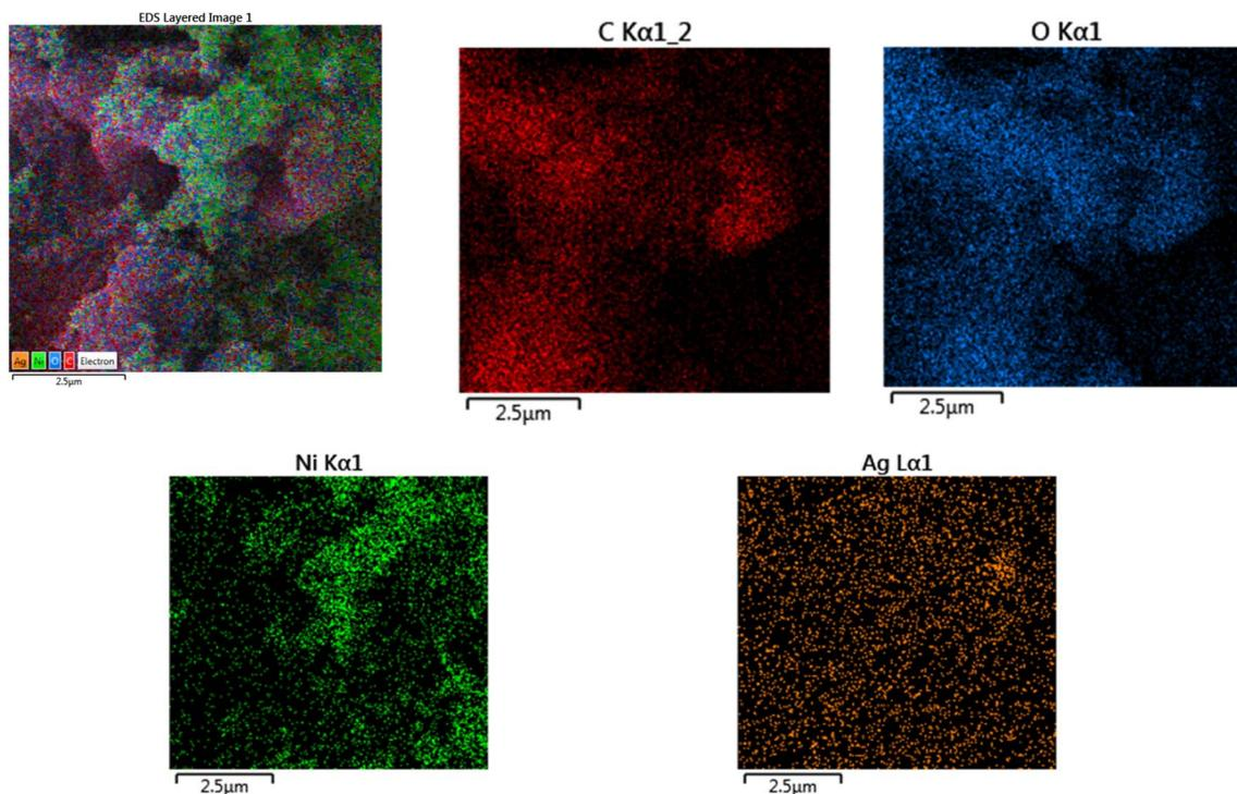
Fig. 5 Mapping FESEM to show elements distribution in rGO/NiO<sub>x</sub>/Ag ternary composite.
