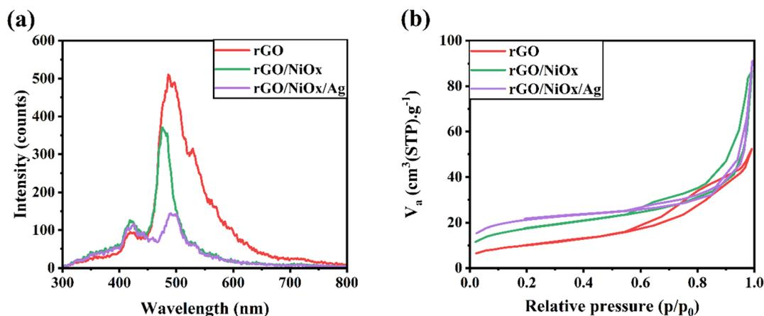
Fig. 8 (a) PL and (b) BET curves of different samples. Excitation wavelength to measure PL spectra was 240 nm.
