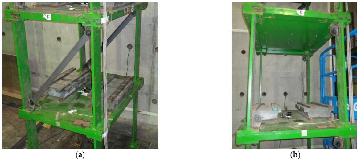
Figure 12. Experimental installation of destructive and non-destructive structures; (a) undamaged condition (no bracing removed); (b) damaged condition (bracing removed).
