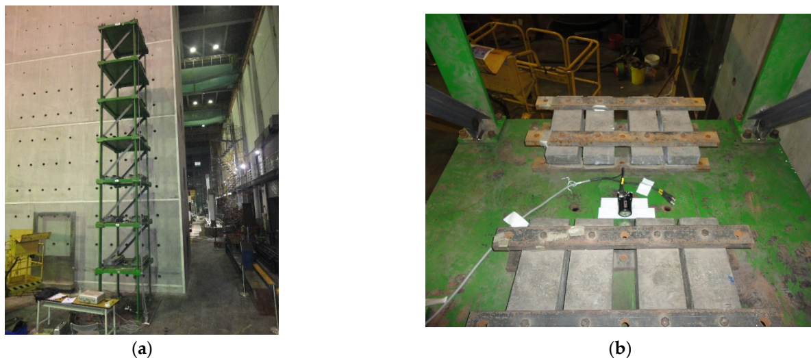
Figure 11. Experimental setup. (a) Seven-story steel frame model; (b) location of the sensor and mass block.
