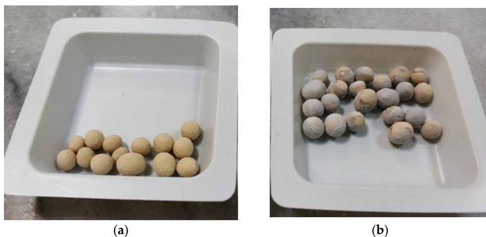
Figure 1. Duranit balls (a) before and (b) after the ZnO deposition.
