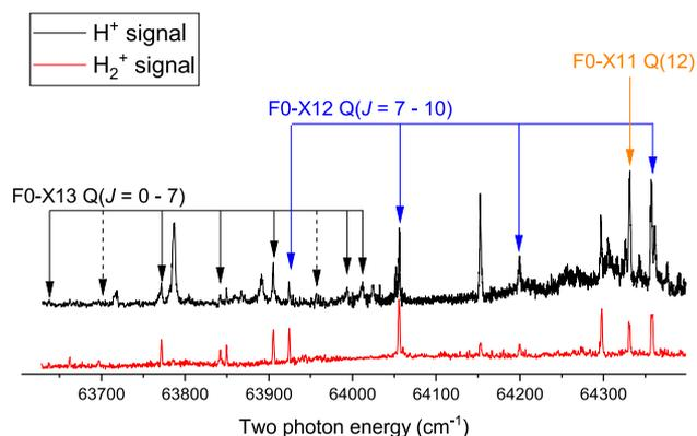
**Figure 3.** Low-resolution overview spectra of the  $\text{F}^1\Sigma_g^+ - \text{X}^1\Sigma_g^+(0,13)$  and  $\text{F}^1\Sigma_g^+ - \text{X}^1\Sigma_g^+(0,12)$  bands probed via one-color 2 + 1 REMPI with a tunable frequency-doubled pulsed dye laser upon  $\text{H}_2$  photolysis. Signals are recorded for both  $\text{H}^+$  and  $\text{H}_2^+$ .
