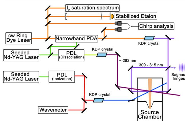
**Figure 1.** Schematic layout of the experimental setup including the three UV-lasers, the calibration units, and the vacuum chambers. For details, see text.
