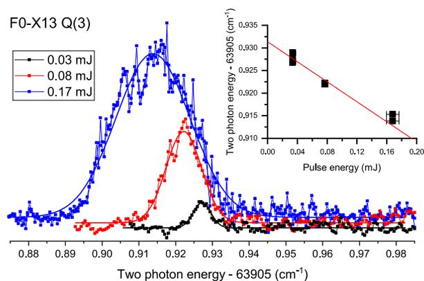
**Figure 4.** Spectra of the F0-X13 Q(3) transition recorded in a two-color 2 + 1' REMPI scheme with tuning of the narrowband frequency-doubled PDA-system with counter-propagating UV-beams. The inset shows the ac-Stark extrapolation to zero power levels.
