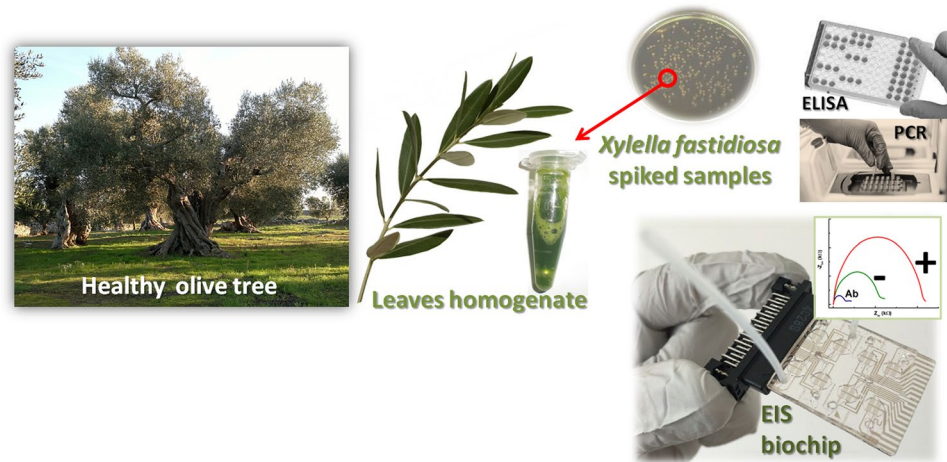
Figure 1. Spiked olive leaves homogenates and real samples (healthy or naturally infected) were tested with two standard techniques and a LOC platform in order to validate the on-chip method for Xylella fastidiosa detection.
