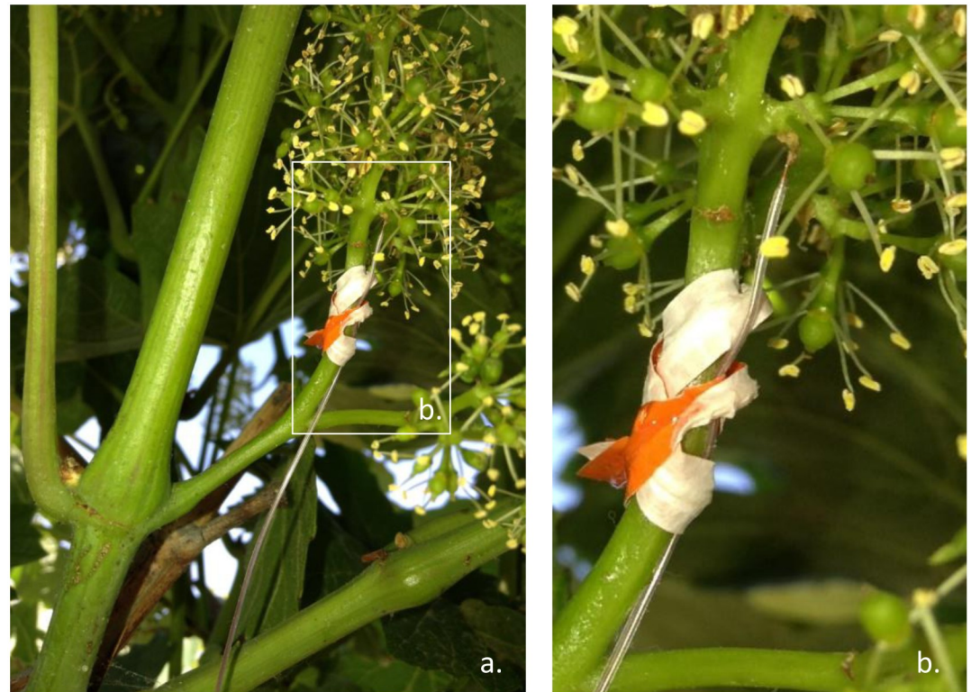
Fig 2. Probe installed to measure air temperature within berry clusters (a). “T type” thermocouples were installed in the rachis, close to the first or second branching point (b).
