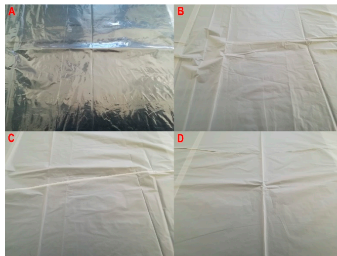
Figure 7. The appearance of the film made at a screw speed of 400 rpm: (A) LDPE, (B) PLA, (C) TPS-C, (D) TPS-P.
