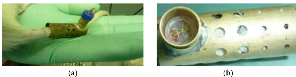
Figure A1. Photos of the pin-port tail cuff in-situ: (a) during study data collection periods; (b) close-up view of the U-shaped loop during recirculation phases (following surgery or between data collection sessions).
