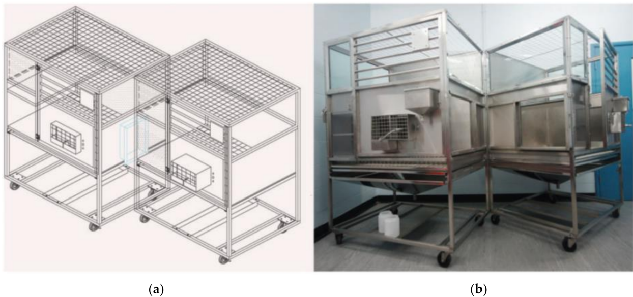
Figure 1. Schematic (a) and photo representation (b) of the dual cage system with a hatch between the two connected cages for pair-housed dogs.
