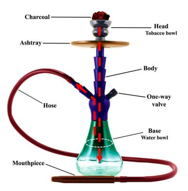
Figure 1. Different parts of one of the most common types of waterpipe smoking device.
