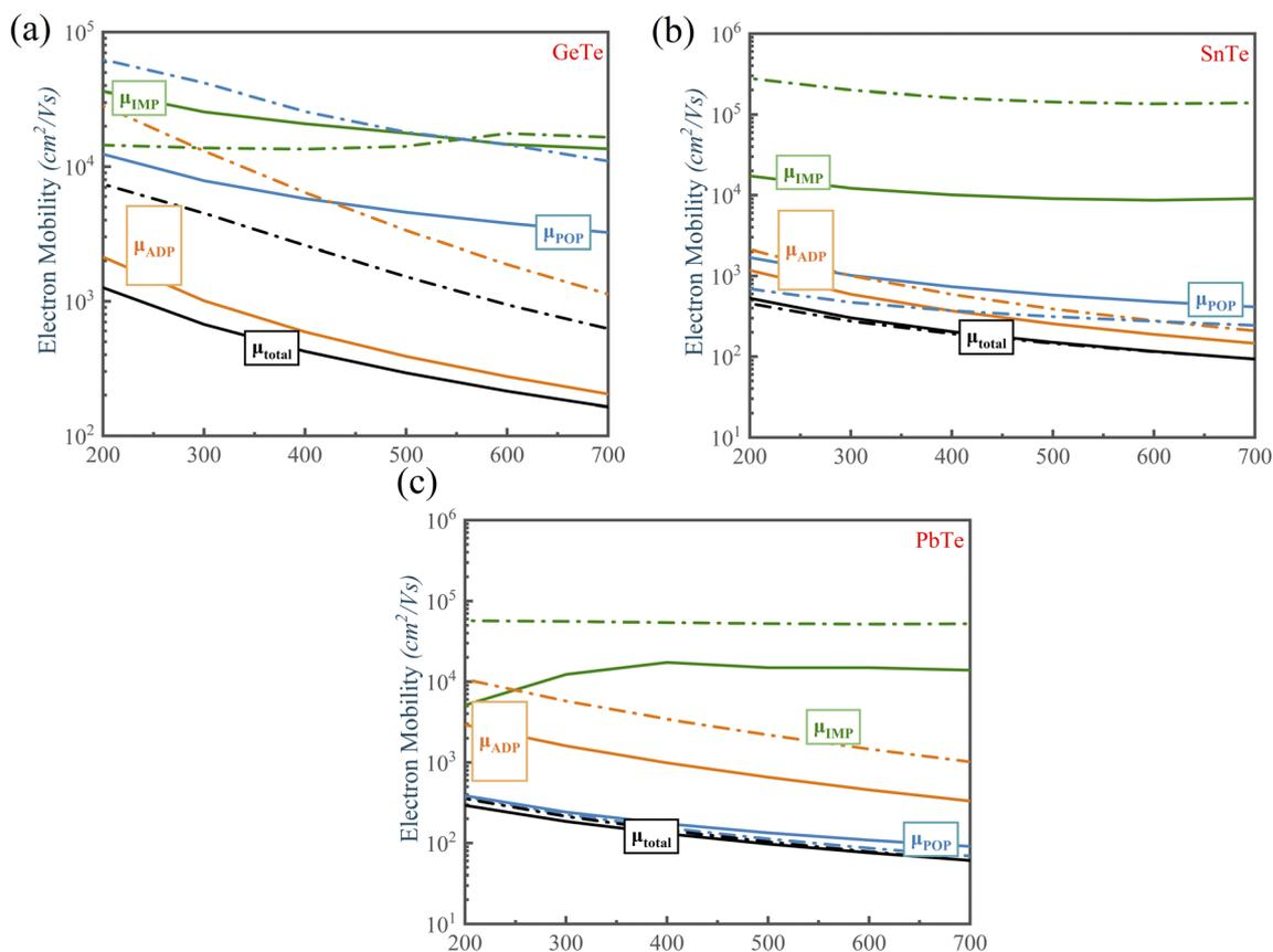
Fig. 7 Electron mobility versus temperature for the doping concentration of  $n = 1 \times 10^{19} \text{ cm}^{-3}$  of n-type MTe. The solid and dashed lines represent the Te coordinate at (0.47, 0.47, 0.47) and (0.50, 0.50, 0.50), respectively. The black line is the calculated mobility including all scattering channels, while the colored lines correspond to the individual contributions of ADP, IMP and POP.
