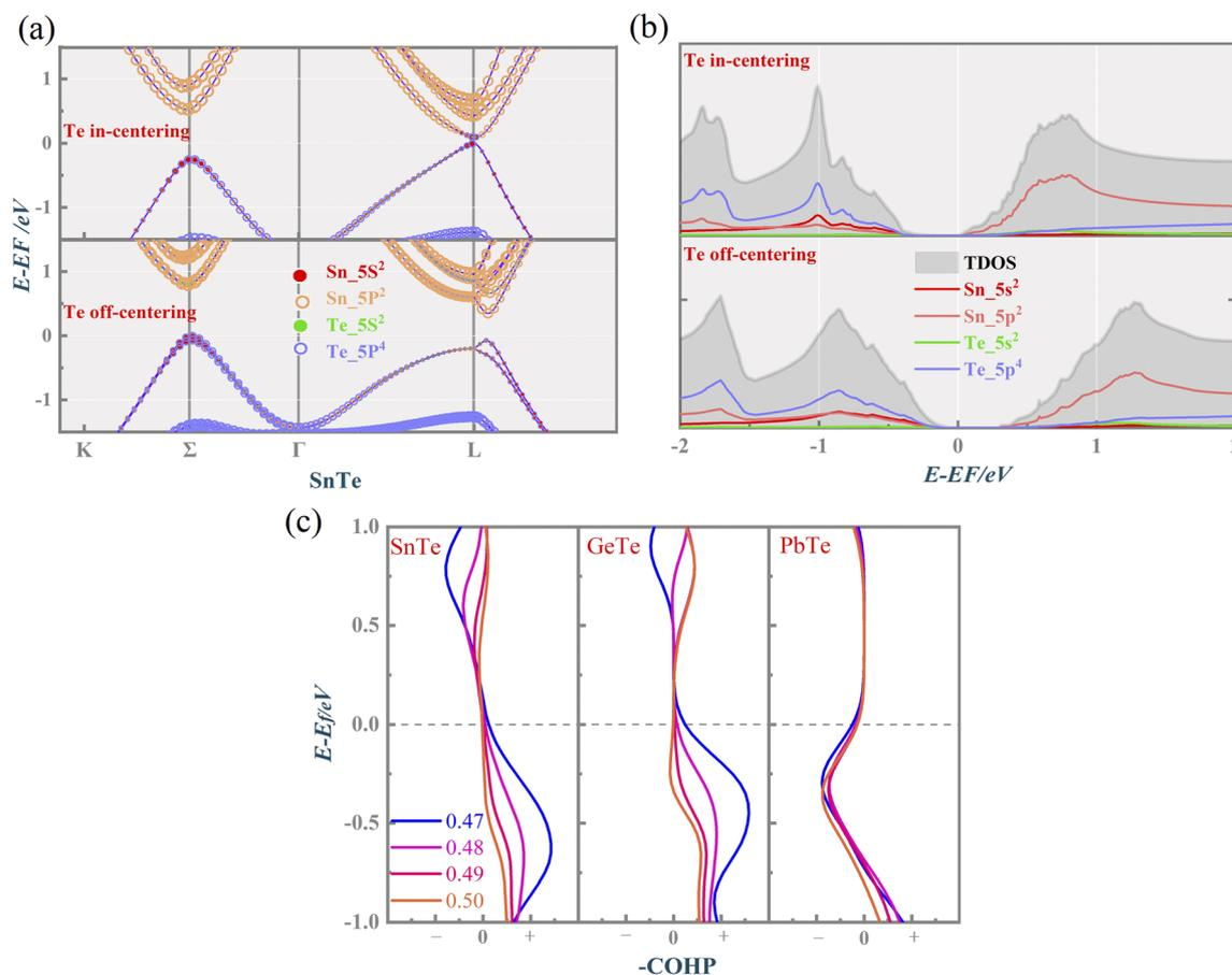
Fig. 3 The calculated (a) PBAND (size of each circle representing the atomic orbital weight) of SnTe, (b) PDOS when the Te atom is located at (0.47, 0.47, 0.47) and (0.50, 0.50, 0.50), respectively, and (c) -COHP of MTe as a function of energy and atomic reciprocal displacement.
