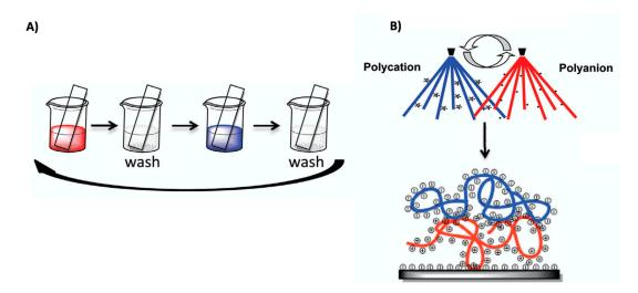
**Figure 2.** Layer-by-layer approach for PEM fabrication: a negatively charged substrate is alternately immersed (**A**) (or sprayed (**B**), for instance) in polycation and polyanion solutions, respectively. Washing steps are to remove unbound polyelectrolytes. Colour-coding: polyanion (blue); polycation (red). Figure adapted with permission from reference [23], copyright © 2020 Elsevier Ltd.
