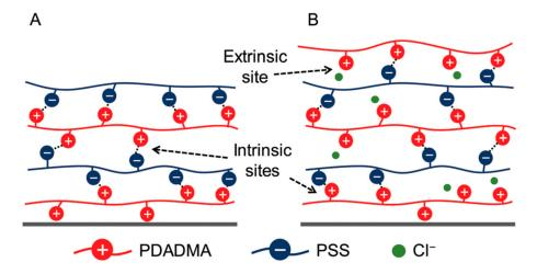
**Figure 6.** (**A**) PSS/PDADMAC multilayers containing only polyion-polyion interactions (i.e., intrinsic charge compensation) and (**B**) the same multilayers but overcharged or overcompensated; also containing extrinsic polyion-counter ion interactions. Figure taken from reference [130], copyright © 2020 Royal Society of Chemistry.
