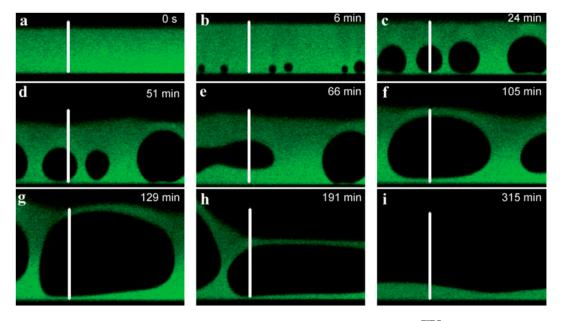
**Figure 14.** Vertical section of PEM observed by CLSM of a (PLL/HA)<sub>50</sub>/PLL<sup>FITC</sup> film built in 0.15 M NaCl and swelled by immersion in solutions of increasing NaCl concentrations, up to 0.48 M, followed as a function of time. The scale bars represent 50  $\mu$ m for (**a**,**b**,**c**), 60  $\mu$ m for (**d**,**e**,**f**), and 80  $\mu$ m for (**g**,**h**,**i**). Figure taken from reference [167], Copyright © 2020 Royal Society of Chemistry.
