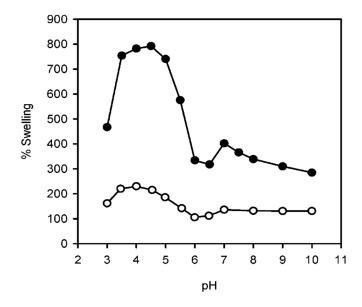
**Figure 10.** Dependence of the degree of swelling for (PLL/HA)<sub>75</sub> films assembled at pH 5 (•) and 9 (•). Figure taken from reference [145], Copyright © 2020 American Chemical Society.
