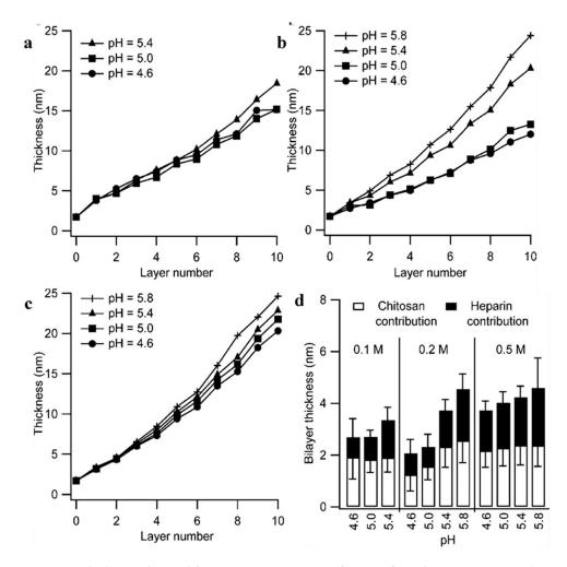
**Figure 9.** PEM thickness obtained from in situ Fourier transform-surface plasmon resonance (FT-SPR) data as a function of layer number and pH for 0.1 M buffer (**a**), 0.2 M buffer (**b**), and 0.5 M buffer (**c**). Odd numbered layers are CHI and even-numbered layers are HS. (**d**) Average incremental bilayer thickness of PEM at different buffer conditions as a function of pH. Figures taken from reference [71], Copyright © 2020 American Chemical Society.
