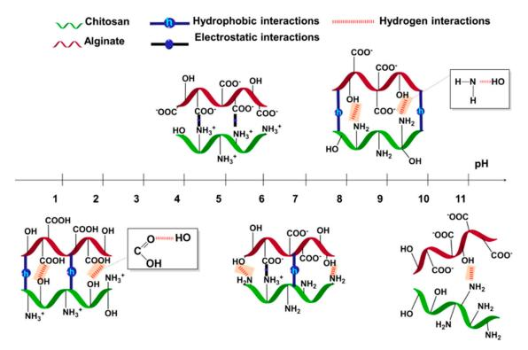
**Figure 11.** Schematic demonstrating the effect of pH on the molecular mobility of multi-layered films, considering the different intermolecular interactions behind them. Figure taken from reference [168], copyright © 2020 American Chemical Society.
