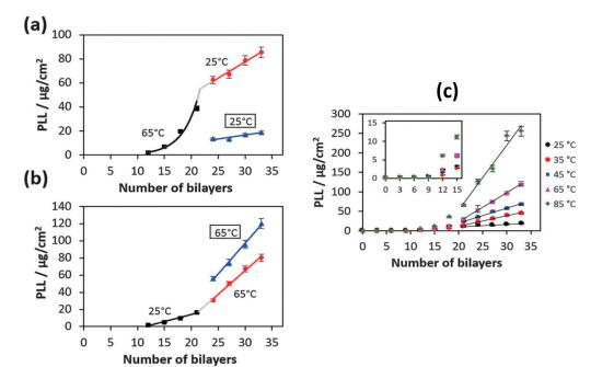
**Figure 8.** (a) Temperature change from 65 °C to 25 °C; (b) Temperature change from 25 °C to 65 °C at the 21st bilayer. The blue triangles represent film preparation at 25 °C and 65 °C without the temperature change after 21 bilayers. (c) Mass coverage of PLL in the HA/PLL film formed at different temperatures. The inset shows the enlarged growth profile until 15 bilayers. Figure taken from reference [141], copyright © 2020 Published by the PCCP Owner Societies.
