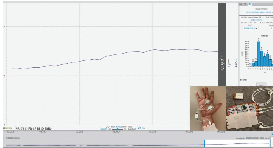
FIGURE 3: Electrodermal activity recorded through the BITalino® platform (in the box).
