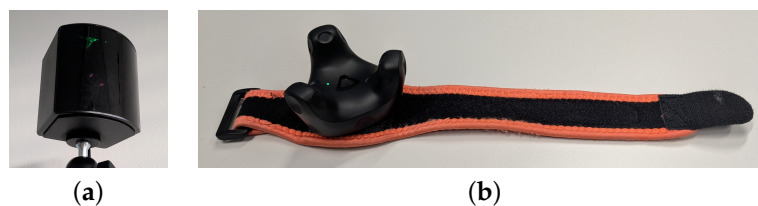
Figure 2. SteamVR Tracking 2.0 components: (a) one of four SteamVR Base Stations 2.0 on a mount, (b) one of two HTC VIVE Trackers (3.0) on a strap.
