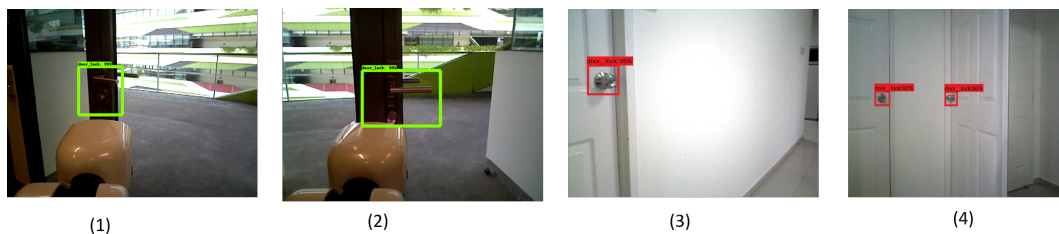
Figure 9. Real-time door-handle detection—(1, 2 Test bed1), (3, 4 Test bed2).
