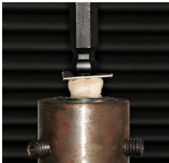
Figure 3. The specimen fixed in the lower compartment of the universal testing machine with the tin foil positioned between the specimen and the metal rod during the fracture test.
