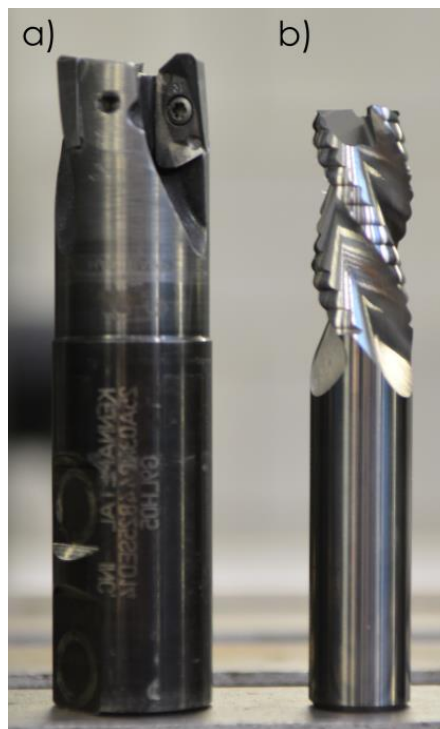
Figure 3. Tools used in studies: (a) Kennametal indexable milling cutter; (b) Sandvik monolithic milling cutter.
