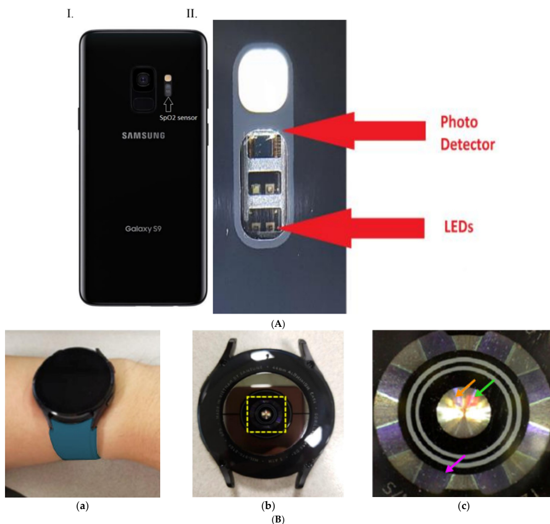
Figure 1. (A): (I) The location of the SpO 2 sensor on the back of the smartphone, making it clear that the sensor is entirely separate from the other phone devices such as the camera. In the expanded view (II), the dedicated photo sensor and LEDs for the pulse oximetry function are shown. The device has a total of 4 LEDs, 2 of which are reserved for future additional functionality. The arrow indicates the 660 nm red and 910 nm infrared LEDs used in this measurement. The photodetector is connected to an extremely low-noise analog channel, allowing for measurement on a broad range of skin colors. (B): The Galaxy Watch 4 (GW4) used in this study. (a): Ideal GW4 placement on the wrist, avoiding the ulnar styloid process of the participants. (b): View of the side of the watch in contact with the skin, showing placement of the light-emitting diodes and photodetector (LED-PD) module (contained in the yellow rectangular area). (c): Magnified view of the LED-PD module with arrows pointing to LEDs and PDs. Photodiodes are located radially, with the purple arrow indicating one of the eight PDs. Infrared LEDs are pointed out by the orange arrow and red LEDs by the green arrow [33].
