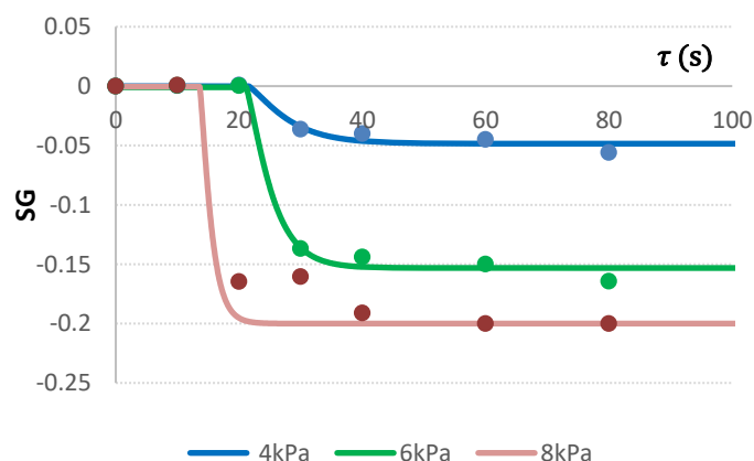
Figure 3. Changes of SG during impregnation of apples at varied vacuum pressures of 4, 6, and 8 kPa using distilled water as the impregnating liquid.
