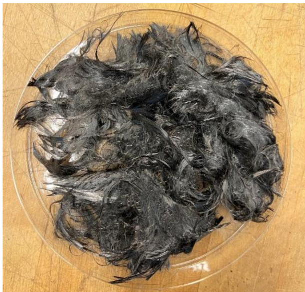
Figure 2. Photograph of recovered fibers after exposing the composite to a 50 wt% acetic acid solution at 300\text{ }^{\circ}\text{C} for 30 min.
