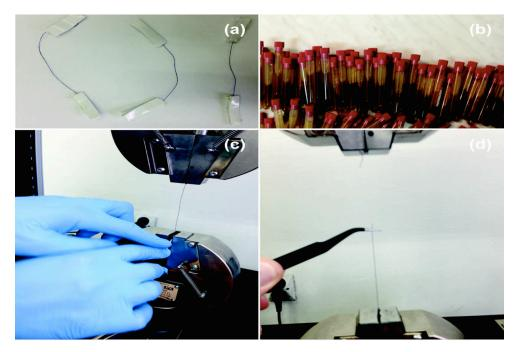
**Figure 1.** Stages of the experiment: (a) sutures before the stretch testing; (b) collected sterile bile and sterile pancreatic juice in cryotubes; (c) INSTRON tensile machine; (d) suture after stretch test.
