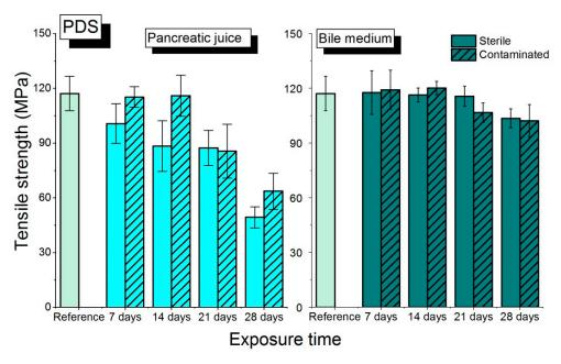
**Figure 5.** The results of the tensile strength of PDS sutures in bile and pancreatic juice, sterile and contaminated, in relation to the exposure time.
