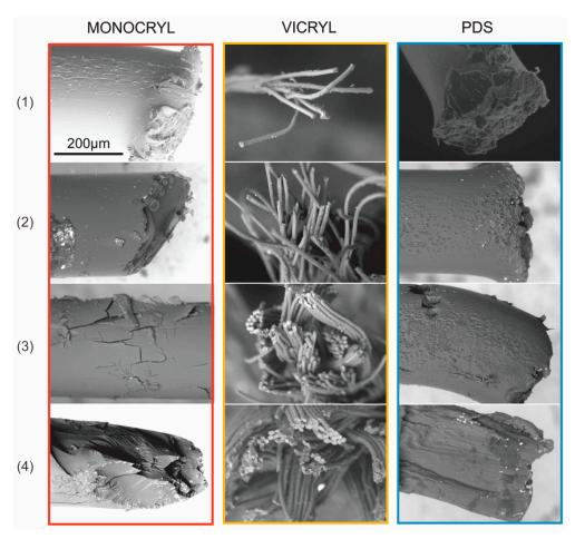
**Figure 6.** Scanning electron microscope images of uncoated sutures on day 21 (for Monocryl and Vicryl in sterile and infected pancreatic juice and bile) and day 28 of the experiment (for all sutures in a saline medium, PDS in all mediums): red box—Monocryl suture; orange box—Vicryl suture; blue box—PDS suture: (1) reference SEM images for the starting sutures (no medium); (2) saline—sterile environment; (3) pancreatic juice—contaminated environment; (4) bile—contaminated environment.
