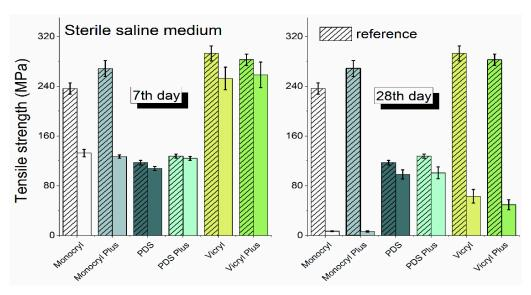
**Figure 2.** Comparison of the tensile strength of each surgical suture examined in sterile saline on days 7 and 28 of the experiment.
