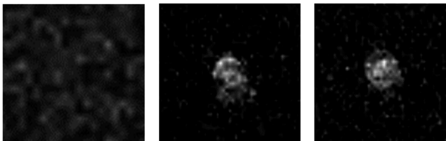
Figure 6. ^{19}\text{F} imaging of a solution (2.5 mM) of probe 11 before (left) and after (middle) SCC7 cell medium incubation. As a control, a solution (right) of F9-PEG-Mal-PEP-DOTA without \text{Gd}^{3+} incorporation was also imaged. The experiments were performed with a homemade surface coil tuned to 281.65 MHz, which is the ^{19}\text{F} resonance frequency at 7 T. A 2D FLASH image was acquired on the probe, with the following acquisition parameters: TE = 3 ms, TR = 100 ms, FOV = 4 \times 4 \text{ cm}^2 , matrix size = 128 \times 128 , slice thickness = 2 mm, and FA = 30 deg.
