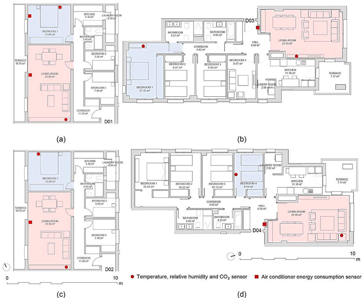
**Fig. 3.** Floor plans of the four monitored dwellings in Seville: (a) D01, (b) D03, (c) D02 and (d) D04. Sensor locations in the monitored rooms are indicated in red. (For interpretation of the references to colour in this figure legend, the reader is referred to the Web version of this article.)
