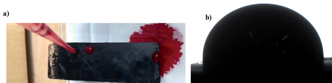
Fig. 7 Photos (a and b) represent the blood repellency and its contact angle with soot slippery surface.
