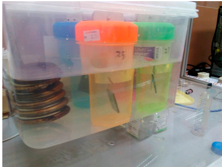
Figure 4. Jars containing specimens in Simulated Body Fluid (SBF) with heating filament for maintaining temperature.
