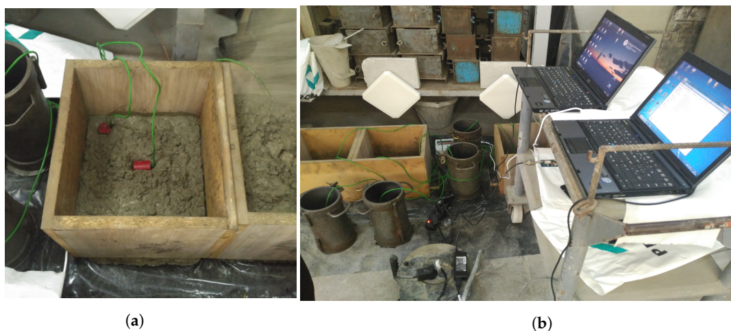
Figure 8. In-field measurement at PROMSA: (a) Location of the embedded RFID sensors and (b) layout of the whole measurement scenario.
