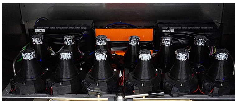
Figure 2. The LiS system equipped with 12 Erlenmeyer flasks in a shaking incubator. The 12 individual LiS vessels are shown in the foreground. The three boxes in the background contain dimmer controls connected to the LEDs and software.
