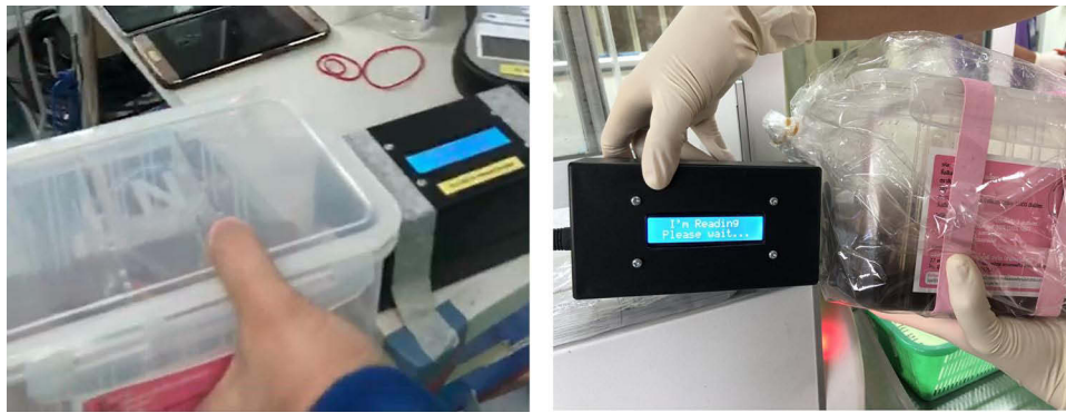
Figure 5 A breast specimen container is scanned by the sensor reader at the OR (left picture), and again by the pathology laboratory (right picture).
