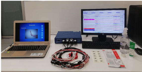
Fig. 3. Measurement system: 4-channel MP36 BIOPAC device and the computer systems.
