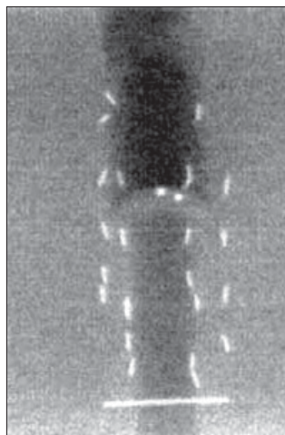
Figure 3b: AP C-arm radiographic image of the gel phantom with 24 seeds
