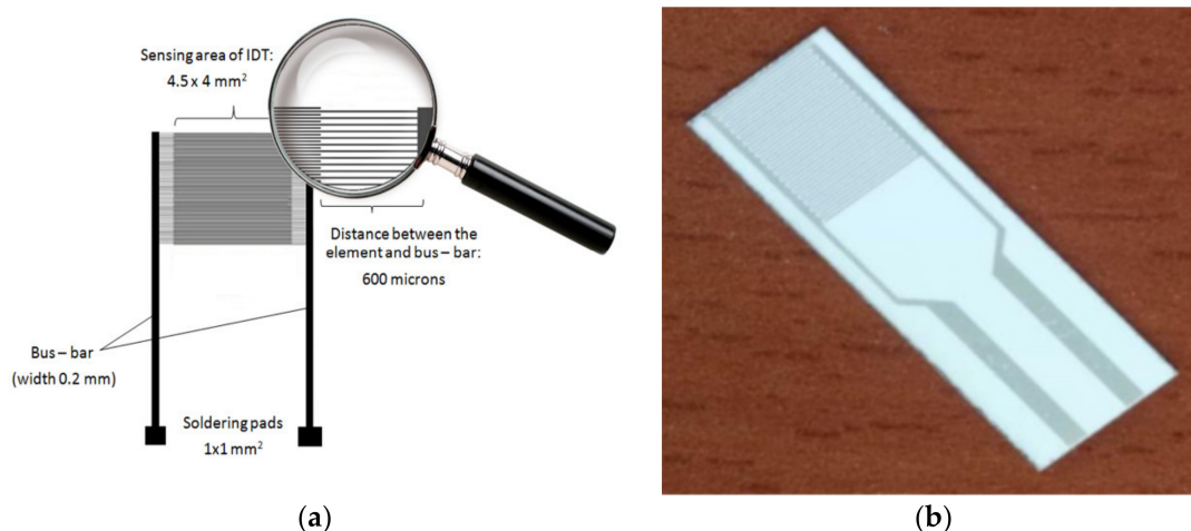
Figure 2. The geometry of: (a) interdigitated transducer (IDT) on rigid substrate (Si/SiO 2 ) and (b) IDT on flexible substrate (polyimide).
