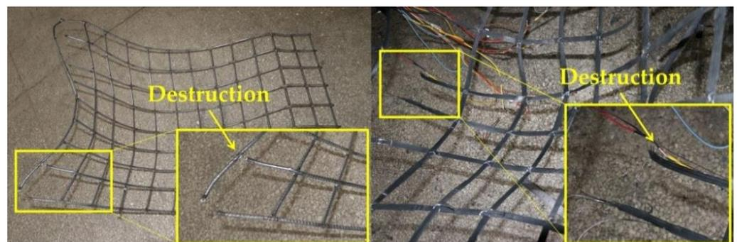
Figure 12. Diagram of mesh damage.
