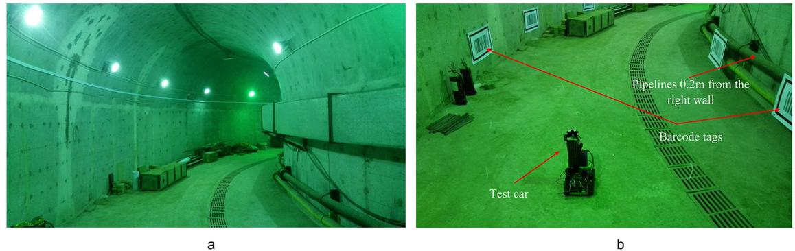
**Fig 23. Test environment of the underground tunnel.** (a) Real figure of the curved tunnel; (b) Deployment graph of the barcode tags;
