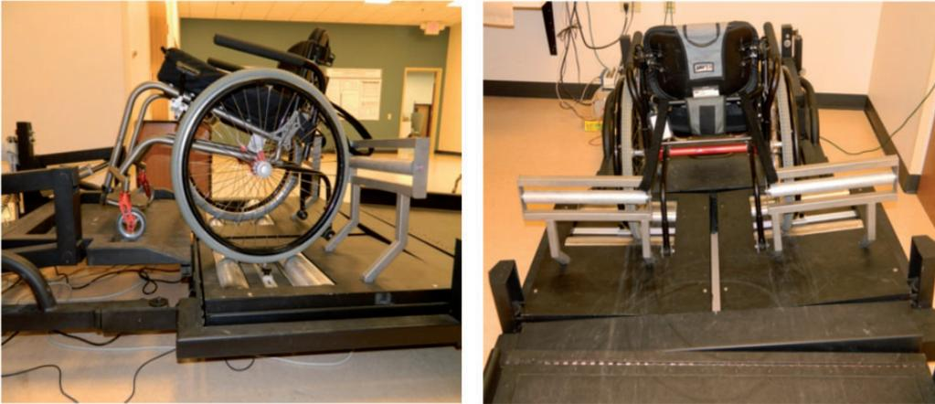
**Figure 1.** The WheelMill System.
