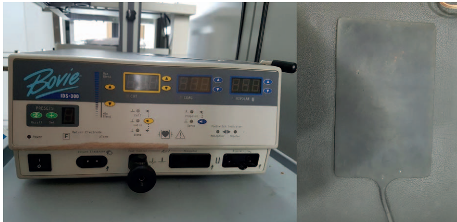
Figure 1. IDS-300 AARON Bovie electrocautery generator and a 7 cm by 10 cm grounding pad made of metal. Grounding pads that do not bend easily are more often used, because of their cheap costs.
