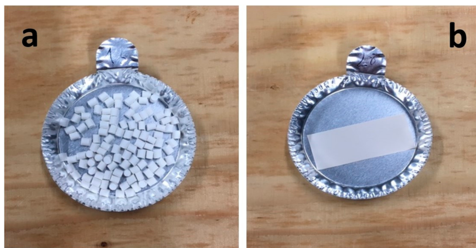
Figure 9. Sample layout for (a) granulates and (b) molded part samples.
